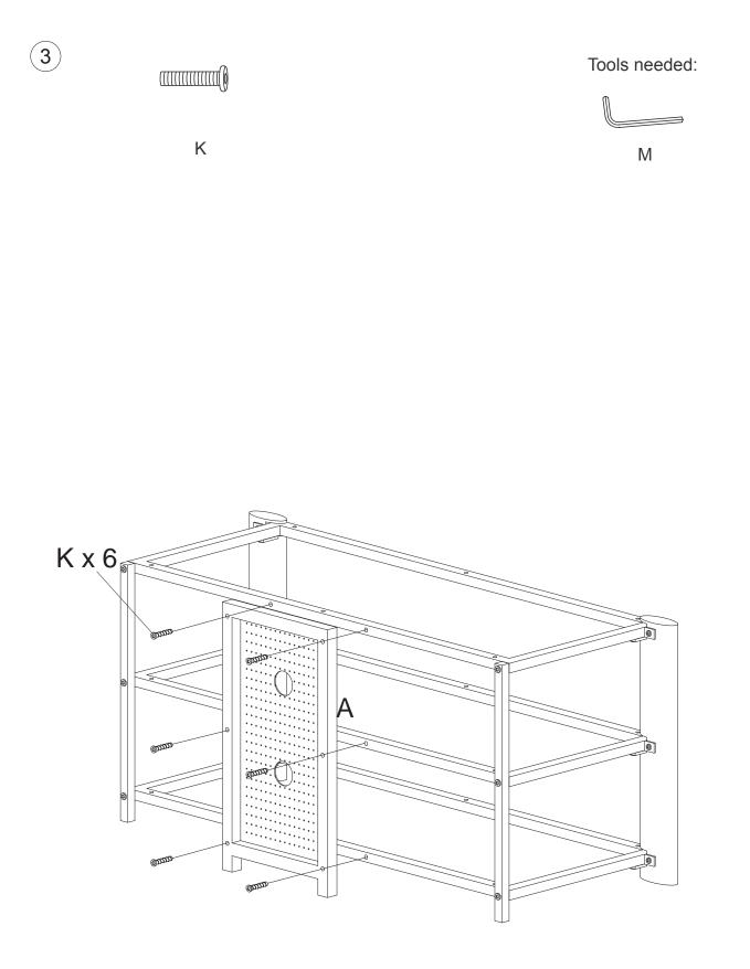
3. Attach back panel (A) to the unit with screws (K).
